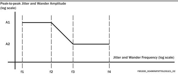
Table 10 Amplitude and Frequency Values for Jitter Tolerance (DS1/E1)
