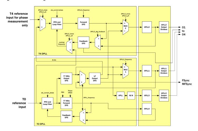
The T4 output APLL is also for multiplying and filtering. The input to the block can come from the T4 forward DFS block or from the T0 path. The input to the T4 output APLL can be programmed to be one of the following:
