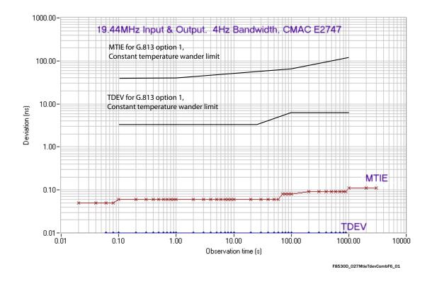
Figure 6 Phase Error Accumulation of TO PLL Output Port in Holdover Mode
