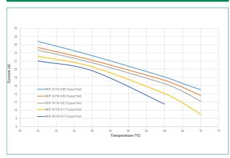
The current versus temperature curve was derived from placing test samples in an oven at  $25^{\circ}\text{C}$ ,  $40^{\circ}\text{C}$ ,  $65^{\circ}\text{C}$ , and  $70^{\circ}\text{C}$ , increasing current flow through the sample at a rate of 0.14/minute and recording the current value when the sample trips.
