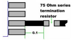
Figure 4. 75 $\Omega$  Series Resistor 0.1 Inches from Pin
