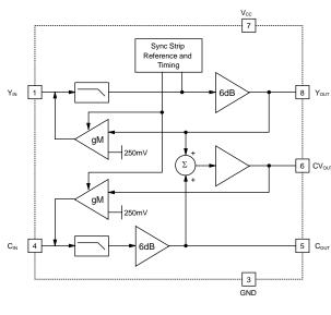
Figure 1. Block Diagram
