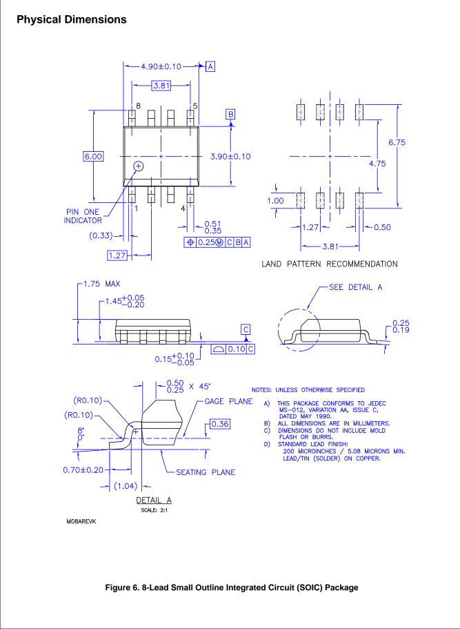
FMS6410B Dual-Channel Video Drivers with Integrated Filters and Composite Video Summer
