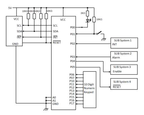
Figure 10: Bidirectional I/O expander application
