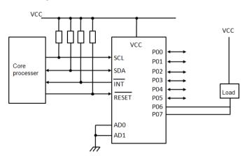
Figure 11: High current-drive load application
