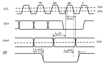
Figure 3: Timing Parameters for INT Signal
