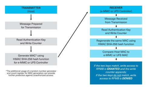
Figure 2: The RPMB Process
