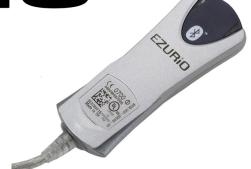
The EZURIO RS232 Adapter allows any device with a standard DB9 RS232 to upgrade to *Bluetooth* wireless connectivity. Using an EZURIO pre-approved module means no further approval required. Combined with our AT style interface this brings versatile adaptation to cable replacement within easy reach.
