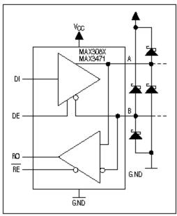
Figure 6. Though expensive, Schottky-diode terminations offer many advantages.
