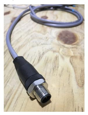
Figure 3. M12 Sensor Connector
