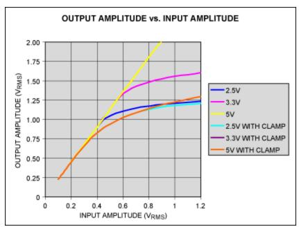
Figure 2. Signal attenuation by the diode network in Figure 1 prevents output clipping by causing a nonlinear transfer of the higher-amplitude inputs. Note that "3.3V with clamp" and "5V with clamp" have the same response and are therefore superimposed. Also, "2.5V" and "3.3V" show compression due to swing limits, even though no clamp is present.
