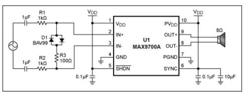
Figure 1. A small-signal diode network limits an amplifier's output voltage.
