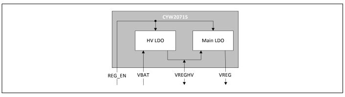
Figure 4. LDO Functional Block Diagram
