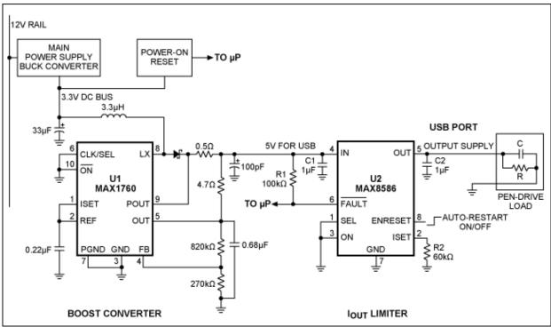
Figure 1. While generating 5V for the USB port, this circuit also limits peak inrush currents at the moment of insertion (at the USB connector), and limits operating current to 500mA as required by the port.
