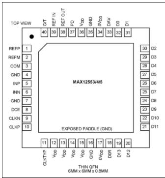
Figure 1. MAX12553, MAX12554, and MAX12555 pinout.
