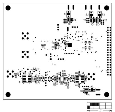
Figure 5. EV Kit bottom-side silkscreen and component placement.
