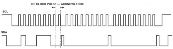
Figure 9: Bus A (0.6V to 5.5V Bus) Waveform
