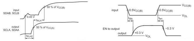
Figure4: Propagation Delay and Enable and disable time
