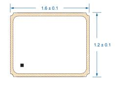
Package: (Scale: none; Dimensions are in mm)
