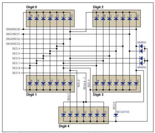
Figure 3. The MAX6958/59 connection to a 4-1/2 digit display.
