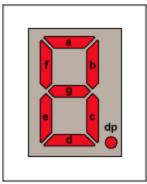
Figure 2. Segment labeling for 7-segment display.
