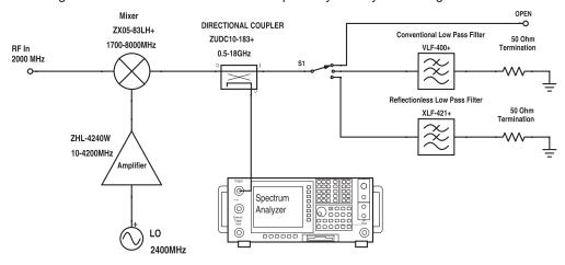
Test block diagram: IF output reflection spectrum with single input frequency
