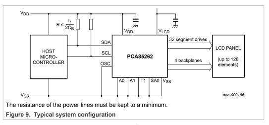
The host microcontroller maintains the 2-line I $^2$ C-bus communication channel with the PCA85262. The internal oscillator is enabled by connecting pin OSC to pin V $_{SS}$ . The appropriate biasing voltages for the multiplexed LCD waveforms are generated internally. The only other connections required to complete the system are the power supplies (V $_{DD}$ , V $_{SS}$ , and V $_{LCD}$ ) and the LCD panel chosen for the application.
