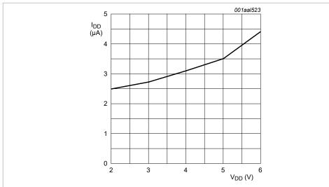
$T_{amb}$  = 30 °C; 1:4 multiplex drive mode;  $V_{LCD}$  = 6.5 V;  $f_{clk(ext)}$  = 1.536 kHz; all RAM written with logic 1; no display connected;  $I^2C$ -bus inactive.
