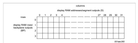
The display RAM bitmap shows the direct relationship between the display RAM column and the segment outputs; and between the bits in a RAM row and the backplane outputs.
