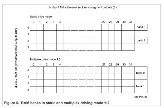
There are two banks; bank 0 and bank 1. <u>Figure 5</u> shows the location of these banks relative to the RAM map. Input and output banks can be set independently from one another with the Bank-select command (see <u>Table 9</u>). <u>Figure 6</u> shows the concept.
