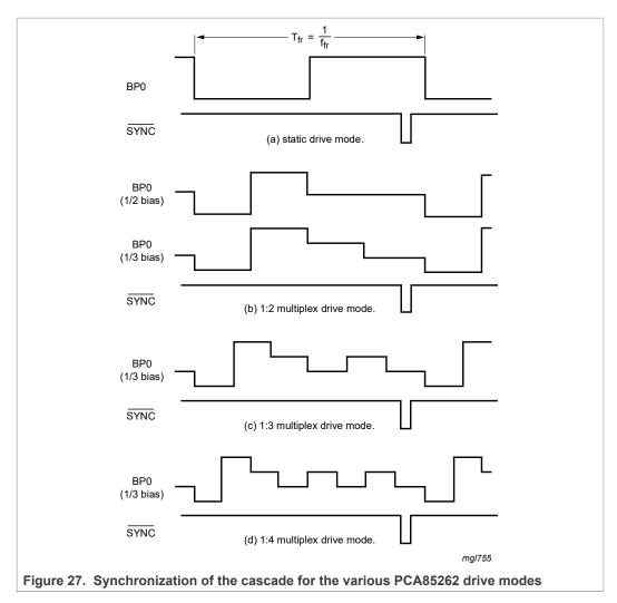
Only one controller but multiple targets are allowed in a cascade. All devices in the cascade have to use the same clock whether it is supplied externally or provided by the controller.
