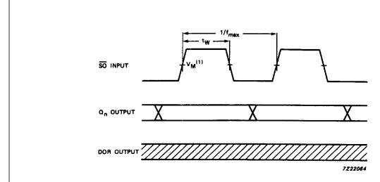
In the high-speed mode, the burst-out rate is determined by the minimum shift-out HIGH and shift-out LOW specifications. The DOR flag is a don't care condition and a SO pulse can be applied without regard to the flag.
