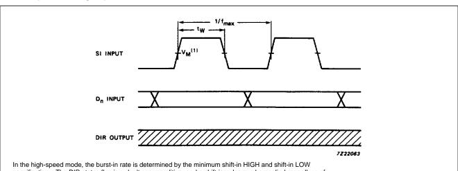
In the high-speed mode, the burst-in rate is determined by the minimum shift-in HIGH and shift-in LOW specifications. The DIR status flag is a don't care condition, and a shift-in pulse can be applied regardless of the flag. A SI pulse which would overflow the storage capacity of the FIFO is ignored.
