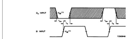
The shaded areas indicate when the input is permitted to change for predictable output performance.
