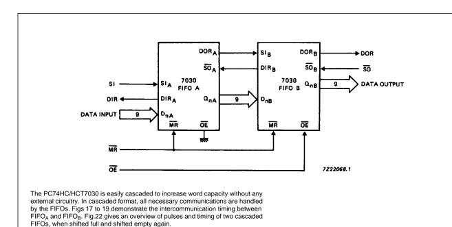
Fig.19 Cascading for increased word capacity; 128 words × 9 bits.
