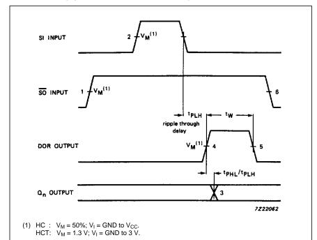
Fig.10 Waveforms showing ripple through delay SI input to DOR output, DOR output pulse width and propagation delay from the DOR pulse to the  $Q_n$  output.
