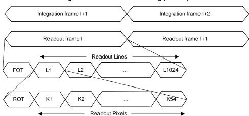
Figure 11. Global Readout Timing (Parallel)
