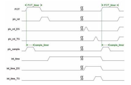
Figure 22. Triple Slope Timing in Slave Mode
