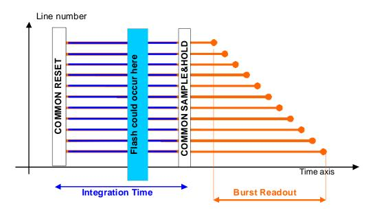
Figure 7. Synchronous Shutter Operation
