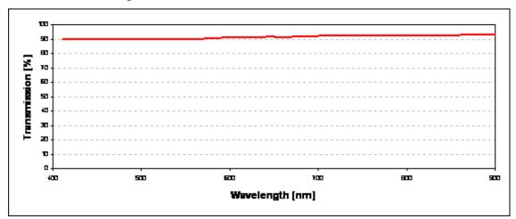
Figure 36. Transmission Characteristics of the Glass lid
