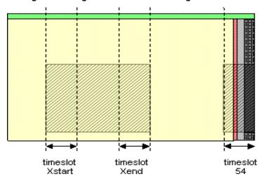
Figure 30. Single Window Not Containing Timeslot 54
