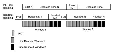
If the X size of the windows are not identical, the integration time in function of the number of lines read presents multiple slopes (proportional to the X size of these windows). Because this can cause confusion when programming the integration time, it is easier to configure all timer registers using the clock cycle configuration instead of the 'line' configuration.
