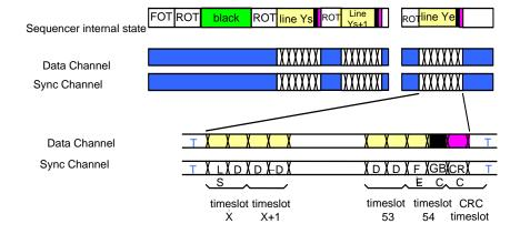
Figure 29. Waveform for Single Window Containing Timeslot 54
