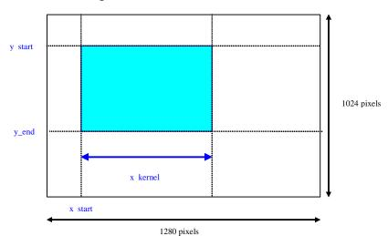
Figure 16. Window Selected for Readout
