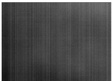
Figure 23. Dark Image Without FPN Correction (5x Amplified)
