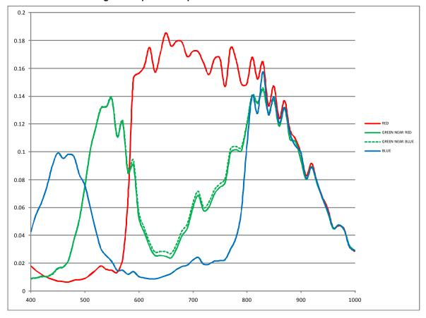
Figure 4. Spectral Response of LUPA 1300-2 Color Sensor
