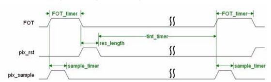
Ensure that the added value of the registers res\_length and tint\_timer always exceeds the number of lines that are read out. This is because the sequencer samples a new image after integration is complete, without checking if image readout is finished. Enlarging res\_length to accommodate for this has no impact on image capture.
