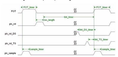
Figure 21. Triple Slope Timing in Master Mode
