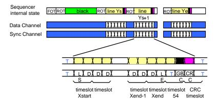
Figure 31. Waveform for Single Window NOT Containing Timeslot 54
