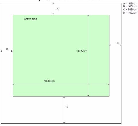
Figure 33. Pixel Active Area Dimensions
