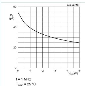
Fig. 29. BC807-25H: Emitter capacitance as a function of emitter-base voltage; typical values
