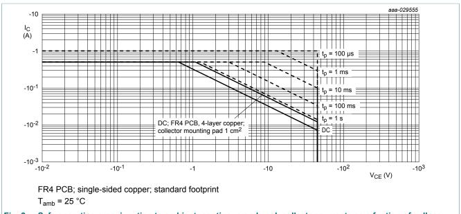
Fig. 2. Safe operating area; junction to ambient; continous and peak collector currents as a funtion of collecoremitter voltage
