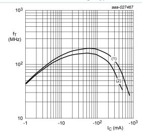
f = 1 MHz  $T_{amb} = 25 \text{ °C}$   $(1) V_{CE} = -5 V$  $(2) V_{CE} = -1 V$
