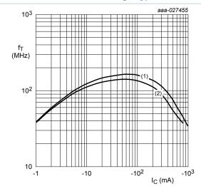
f = 1 MHz $T_{amb}$  = 25 °C (1)  $V_{CE} = -5 V$ (2)  $V_{CE} = -1 V$
