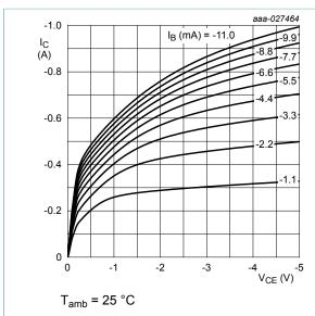
Fig. 39. BC807-40H: Collector current as a function of collector-emitter voltage; typical values
