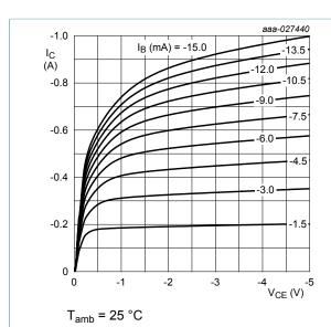
Fig. 15. BC807-16H: Collector current as a function of collector-emitter voltage; typical values
