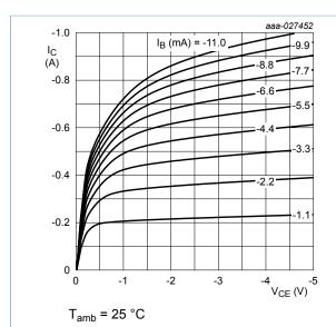
Fig. 27. BC807-25H: Collector current as a function of collector-emitter voltage; typical values
