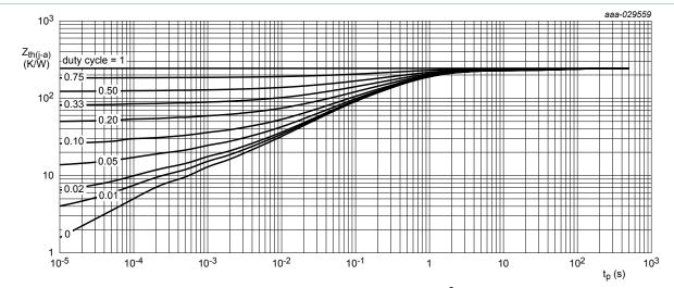
FR4 PCB; 4-layer copper; tin-plated; mounting pad for collector 1 cm<sup>2</sup>
