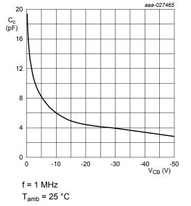
Fig. 40. BC807-40H: Collector capacitance as a function of collector-base voltage; typical values
