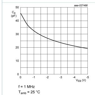
Fig. 41. BC807-40H: Emitter capacitance as a function of emitter-base voltage; typical values
