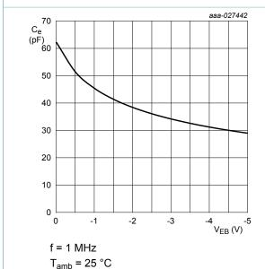
Fig. 17. BC807-16H: Emitter capacitance as a function of emitter-base voltage; typical values
