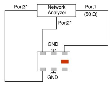
\*Impedance for ports 2 and 3=1/2(Balanced impedance)
