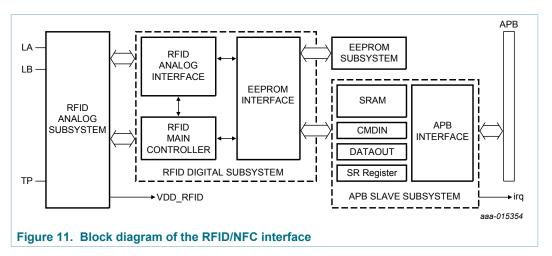
The CMDIN, DATAOUT, Status Register (SR), and SRAM are mapped in the user memory space of the RFID core. The RFID READ and WRITE commands allow wireless communication to this shared memory.
