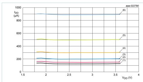
Plot of I<sub>DD</sub> / V<sub>DD</sub> when ARM running a while - 1 loop in Normal mode, no NFC field present.
