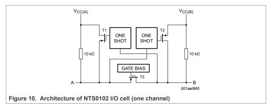
The NTS0102 is a "switch" type voltage translator, it employs two key circuits to enable voltage translation:
