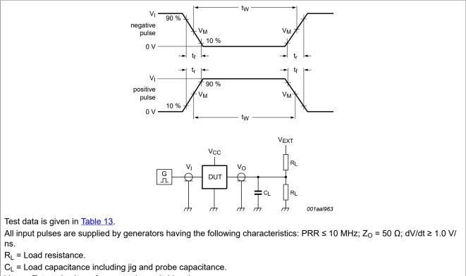
$V_{EXT}$  = External voltage for measuring switching times.
