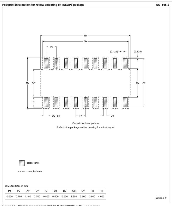
Figure 18. PCB footprint for SOT505-2 (TSSOP8); reflow soldering
