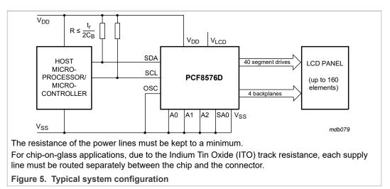
The host microcontroller maintains the 2-line l<sup>2</sup>C-bus communication channel with the PCF8576D. The internal oscillator is enabled by connecting pin OSC to pin V<sub>SS</sub>. The appropriate biasing voltages for the multiplexed LCD waveforms are generated internally. The only other connections required to complete the system are to the power supplies (V<sub>DD</sub>, V<sub>SS</sub>, and V<sub>LCD</sub>) and the LCD panel chosen for the application.
