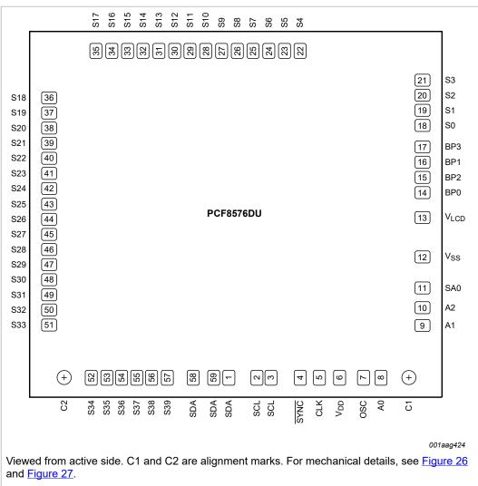
Figure 3. Pinning diagram for PCF8576DU (bare die)
