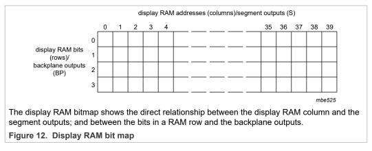
When display data is transmitted to the PCF8576D, the received display bytes are stored in the display RAM in accordance with the selected LCD drive mode. The data is stored as it arrives and depending on the current multiplex drive mode the bits are stored singularly, in pairs, triples, or quadruples. To illustrate the filling order, an example of a 7-segment display showing all drive modes is given in Figure 13; the RAM filling organization depicted applies equally to other LCD types.
