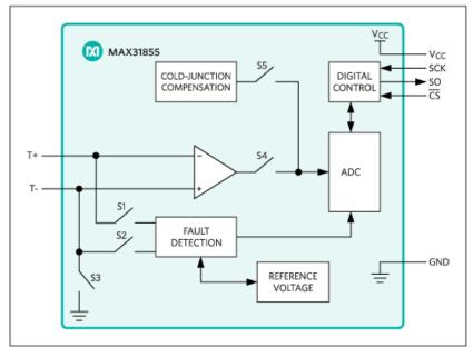
Figure 1. A complete thermocouple-to-digital converter includes cold-junction compensation and fault detection.
