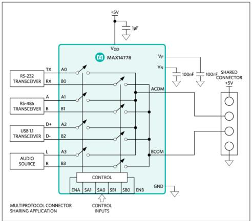
Figure 4. On-chip charge pumps allow the MAX14778 to implement multiprotocol sharing, amongst other functions, with signals as large as ±25V while operating on a single 3.0V to 5.5V supply.
