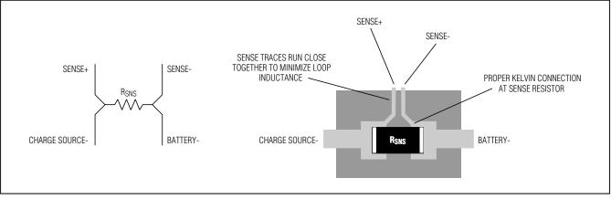
Figure 7. Sense Resistor Connection Layout
