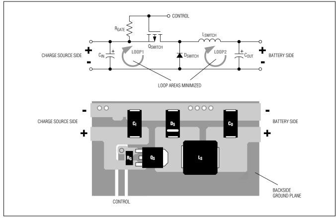
Figure 6. Switching Circuit with Example Layout
