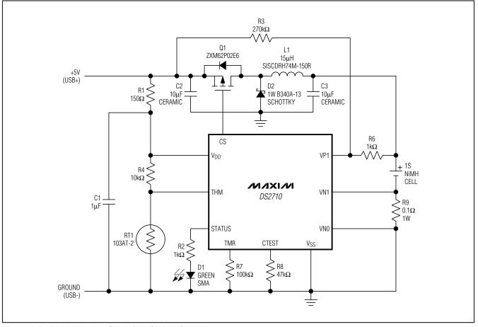
Figure 5. Typical Application Circuit for USB Port Charging
