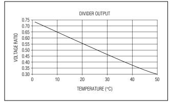
Figure 4. Ratio of THM Pin to V<sub>DD</sub> Pin Over Temperature
