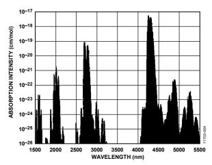
Figure 4. Absorption Spectrum of Carbon Dioxide (CO<sub>2</sub>)
