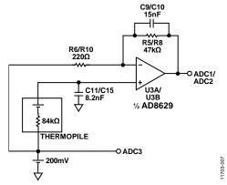
Figure 7. Thermopile Driver Equivalent Circuit, G = 214.6
