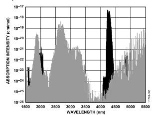
Figure 5. Absorption Spectrum of Carbon Dioxide Overlaid with Water
