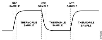
Figure 10. Timing of NTC and Thermopile Sampling and Lamp Chopping
