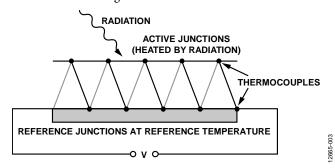
Figure 3. Thermopile Constructed of Multiple Thermocouples
