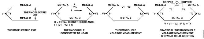
Figure 2. Thermocouple Principles
