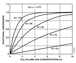
Figure 6. Typical Fractional Absorbance for kl = 4.5, 10, 25, 50, 115
