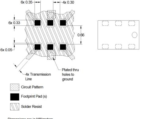
Dimensions are in Millimeters Mounting Footprint
