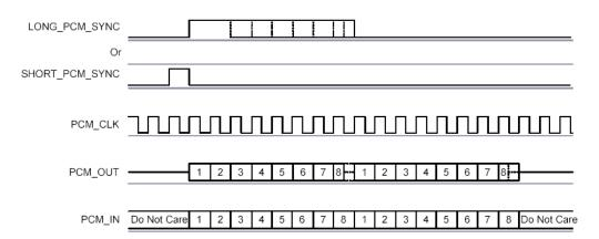
Figure 29: Multi-slot Operation with Two Slots and 8-bit Companded Samples
