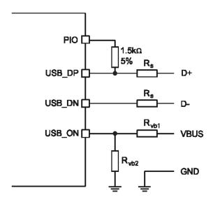
Figure 21: USB Connections for Self-Powered Mode
