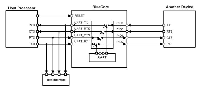
Figure 20: UART Bypass Architecture
