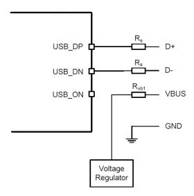
Figure 23: USB Connections for Bus-Powered Mode
