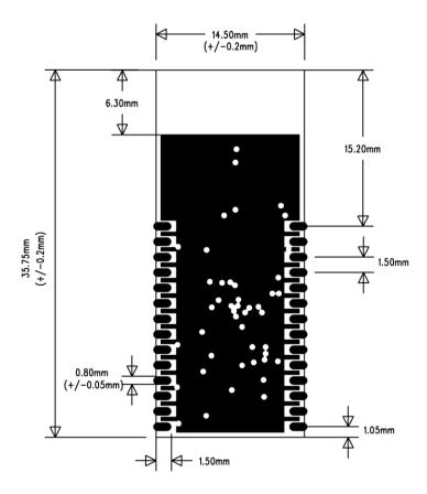
Figure 9: Physical dimensions (top view)
