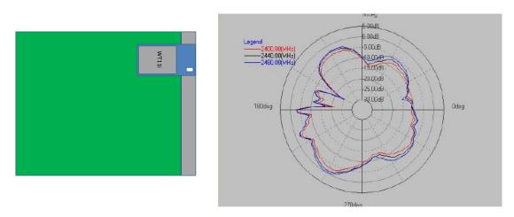
Figure 6: Antenna radiation pattern in the WT11 evaluation kit
