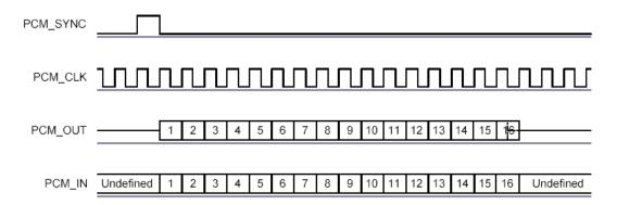
Figure 28: Short Frame Sync (Shown with 16-bit Sample)
