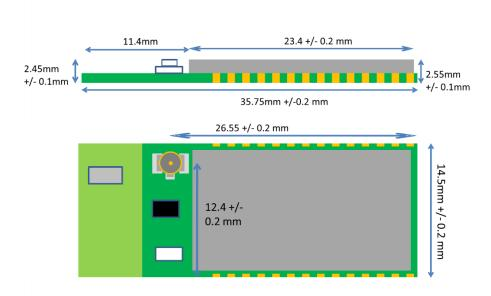
Figure 11: Dimensions of WT11u-E
