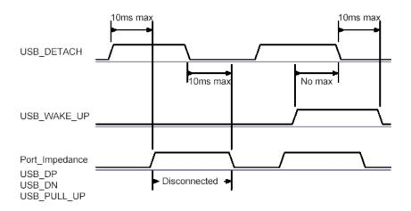
Figure 24: USB\_Detach and USB\_Wake\_Up Signals
