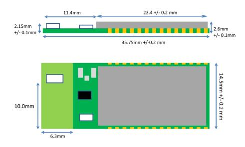
Figure 10: Dimensions of WT11u-A
