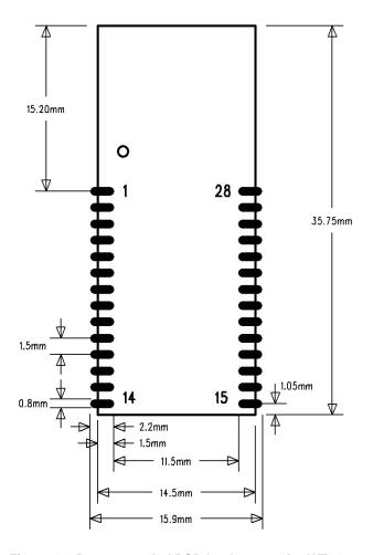
Figure 14: Recommended PCB land pattern for WT11u
