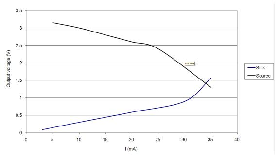
Figure 2: WT11u PIO Current Drive Capability
