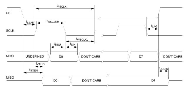
Figure 34. SPI timing characteristics
