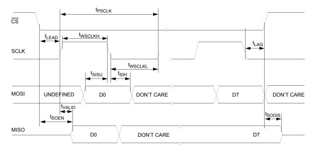
Figure 13. SPI timing characteristics
