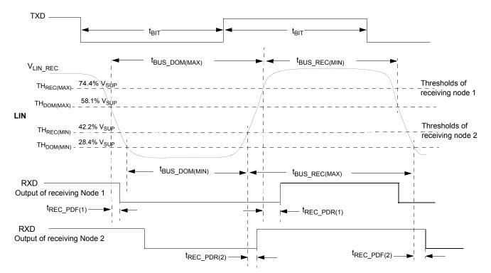
Figure 7. LIN timing measurements for normal slew rate
