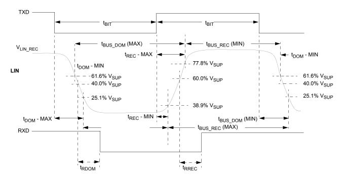
Figure 29. LIN timing measurements for slow slew rate
