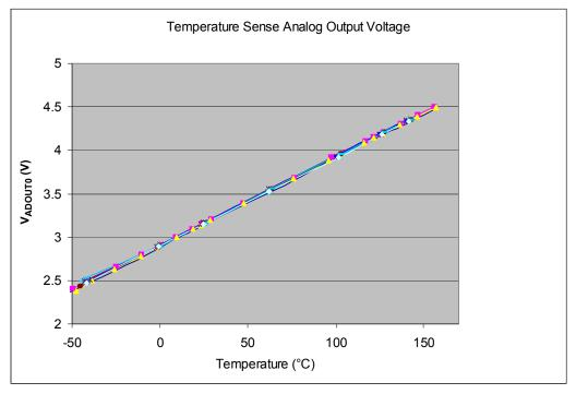
Figure 16. Temperature sense gain
