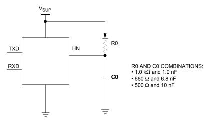
Figure 27. Test circuit for LIN timing measurements
