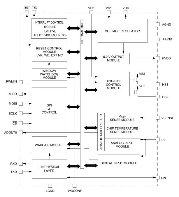
Figure 2. 33910 simplified internal block diagram
