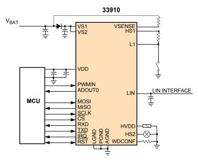
Figure 1. 33910 simplified application diagram
