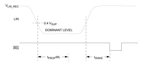
Figure 32. LIN wake-up stop mode timing
