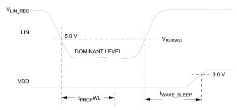
Figure 10. LIN wake-up sleep mode timing
