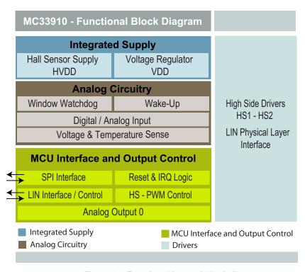
Figure 35. Functional internal block diagram
