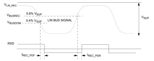
Figure 9. LIN receiver timing
