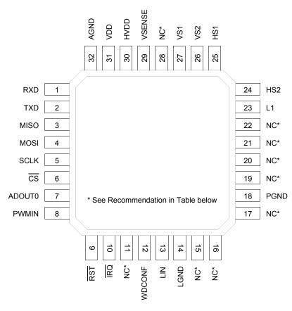
Figure 3. 33910 pin connections
