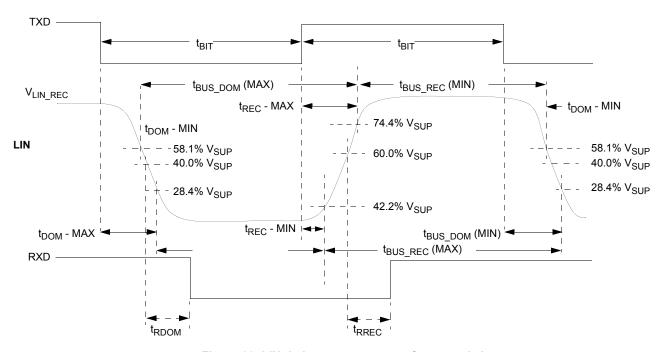
Figure 28. LIN timing measurements for normal slew rate
