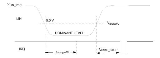
Figure 11. LIN wake-up stop mode timing
