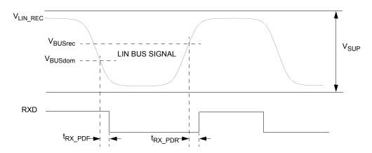
Figure 30. LIN receiver timing
