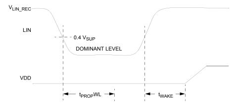
Figure 31. LIN wake-up sleep mode timing
