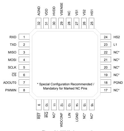
Figure 24. 33910 pin connections
