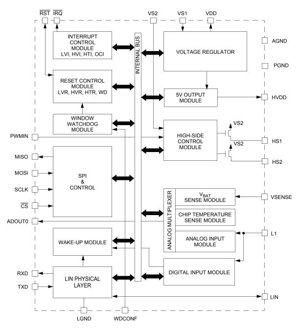
Figure 23. 33910 Simplified internal block diagram
