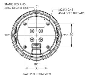
Figure 7, Sweep Mounting Features (all dimensions in mm)
