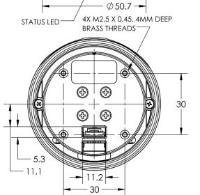
ALL DIMENSIONS ARE IN MM, DRAWINGS ARE NOT TO SCALE Figure 1, Sweep Dimension Drawing
