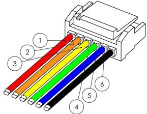
Figure 5, Sweep Pigtail Cable Connector Detail
