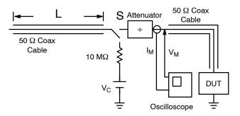
Figure 6. Simplified Schematic of a Typical TLP System
