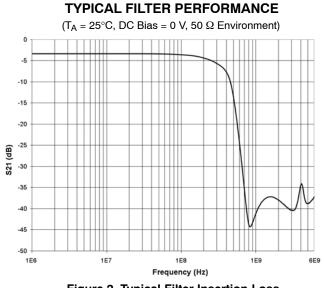
Figure 2. Typical Filter Insertion Loss
