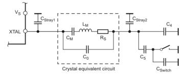
Using  $C_4 = 9.2pF \pm 2\%$ ,  $C_5 = 6.8pF \pm 5\%$ , a switch port with  $C_{Switch} = 3pF \pm 10\%$ , stray capacitances on each side of the crystal of  $C_{Stray1} = C_{Stray2} = 1pF \pm 10\%$ , a parallel capacitance of the crystal of  $C_0 = 3.2pF \pm 10\%$  and a crystal with  $C_M = 13fF \pm 10\%$ , an FSK deviation of  $\pm 21kHz$  typical with worst case tolerances of  $\pm 16.3kHz$  to  $\pm 28.8kHz$  results.
