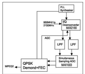
Figure 8. A commercial satellite-receiver system employs simultaneous sampling of the I and Q signals.
