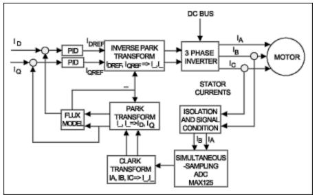
Figure 4. This simplified block diagram illustrates sensorless field-oriented motor control.
