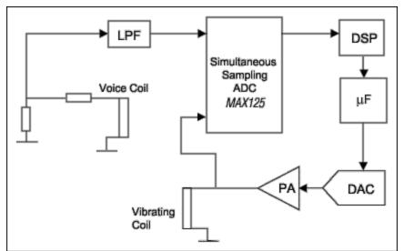
Figure 7. This simplified block diagram shows a typical Coriolis-based mass-flow meter.
