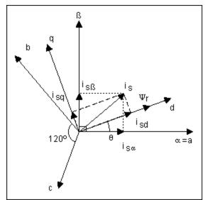
Figure 5. This vector diagram depicts the coordinate transformations necessary in field-oriented control (FOC).
