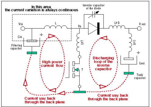
Figure 5. When the main switching transistor (T) turns off, the diode capacitance discharges as shown.
