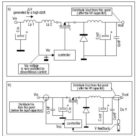
Figure 8. Unwanted common-impedance coupling (a) is prevented by the connections shown in (b).
