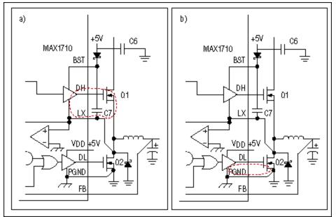
Figure 3. The dotted lines indicate heavy current flow in the gate-discharge (turn-off) paths for Q1 (a) and Q2 (b).
