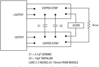
Figure 3. Measuring Output Ripple and Noise (PARD)
