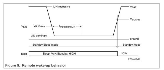
The remote wake-up request is communicated to the microcontroller in Standby mode by a continuous LOW level on pin RXD.
