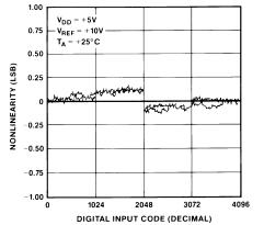
Figure 7. Nonlinearity vs. Code (DAC A and B are Superimposed)
