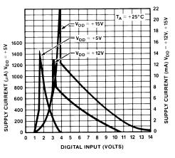
Figure 13. Supply Current vs. Logic Input Voltage
