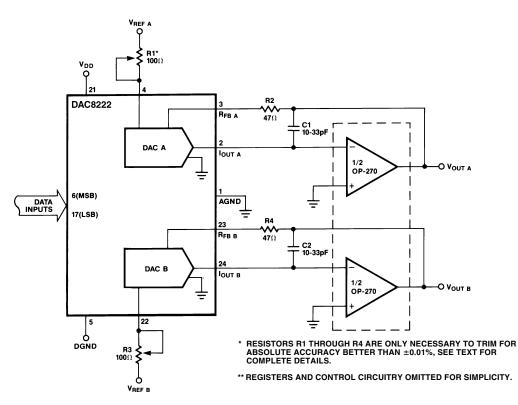
Figure 24. Unipolar Configuration (Two-Quadrant Multiplication)
