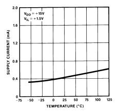
*Figure 12. Supply Current vs. Temperature*
