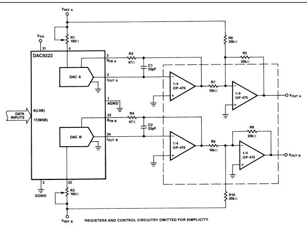
Figure 25. Bipolar Configuration (Four-Quadrant Multiplication)
