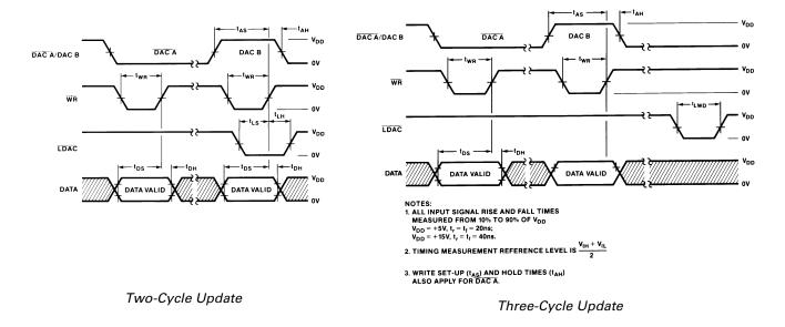
Figure 23. Write Cycle Timing Diagram
