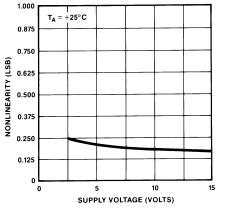
Figure 6. Nonlinearity vs. V<sub>DD</sub>
