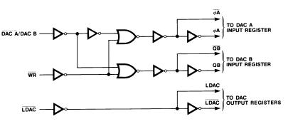
Figure 22. Input Control Logic
