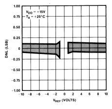
Figure 3. Differential Nonlinearity vs. V<sub>REF</sub>
