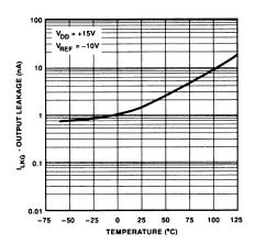
Figure 15. Output Leakage Current vs. Temperature
