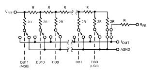
Figure 19. Simplified Single DAC Circuit Configuration. (Switches Are Shown for All Digital Inputs at Zero)
