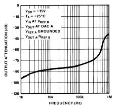
Figure 16. Analog Crosstalk vs. Frequency
