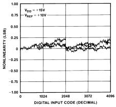
Figure 8. Nonlinearity vs. Code at T<sub>A</sub>  $= -55^{\circ}C$ ,  $+25^{\circ}C$ ,  $+125^{\circ}C$  for DAC A and B (All Superimposed)
