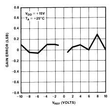
Figure 9. Absolute Gain Error Changes vs. V<sub>REF</sub>
