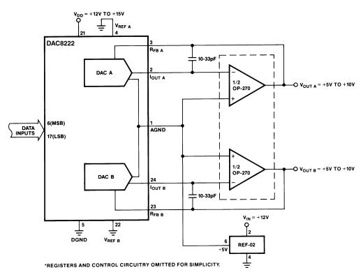
Figure 26. Single Supply Operation (Current Switching Mode)
