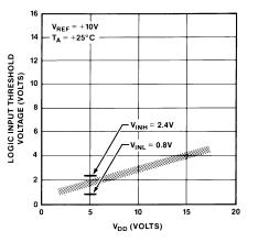
Figure 11. Logic Input Threshold Voltage vs. Supply Voltage (V<sub>DD</sub>)
