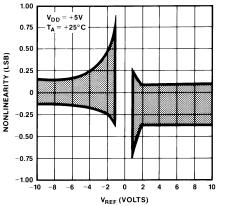
Figure 4. Nonlinearity vs. V<sub>REF</sub>
