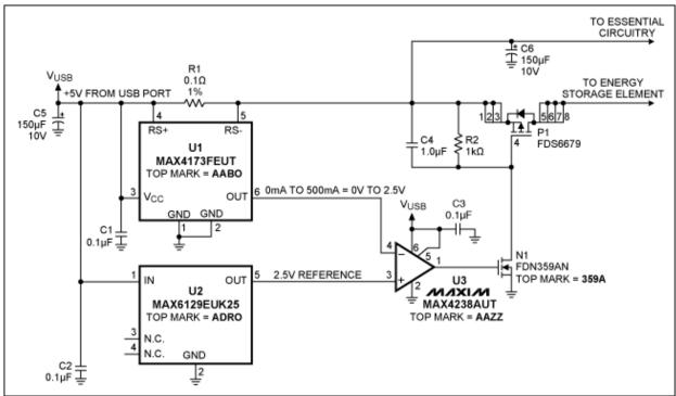
storage element (**Figure 3**) by ensuring that the sum of battery and essential-circuitry currents never exceeds the maximum allowed for a USB high-power device (500mA).
