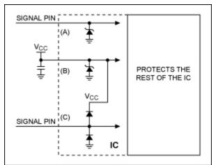
Figure 3. Typical ESD protection structures.
