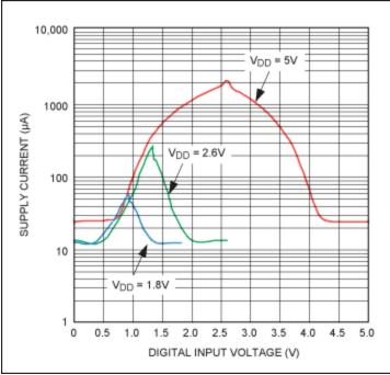
Figure 2. Voltage on a CMOS input pin versus power-supply current. Data are for the MAX5391 digital potentiometer.
