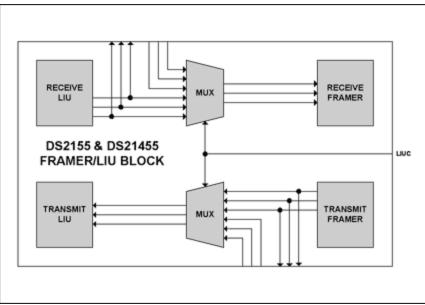
Figure 1. Simplified block diagram of DS2155 transceiver.
