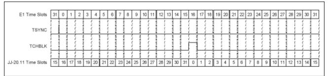
Figure 3. Transmit-side backplane timing.
