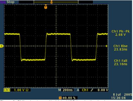
Figure 6. CMI pulse transmitted into  $110\Omega$  termination load.
