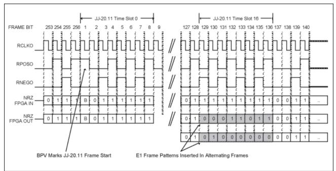
Figure 2. Receive synchronization framing and bit position information.
