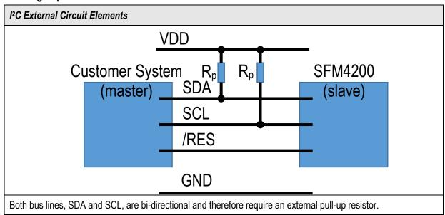
Communication between a master and the SF05 sensor system runs via the digital I<sup>2</sup>C-interface. For detailed specifications of the I<sup>2</sup>C protocol, please refer to the document "The I<sup>2</sup>C-Bus Specification, Version 2.1, January 2000" from NXP (http://www.nxp.com/products/interface\_control/i<sup>2</sup>c).
