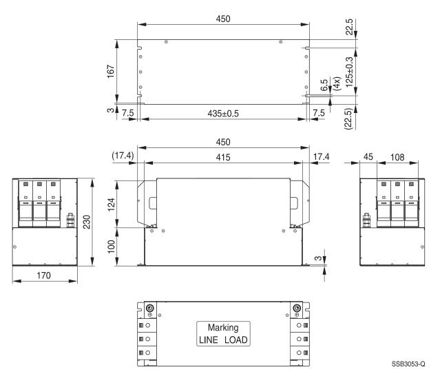
General tolerances according to ISO 2768-cL Dimensions in mm
