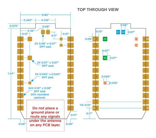
In addition to the 24 pins around the outside of the Photon, there are 7 pads on the bottom the Photon PCB that can be used to connect to extra signals: RGB LED outputs, SETUP button, SMPS enable line and USB D+/D-. Photon Pins #25-31 are described in the Pin out diagrams.
