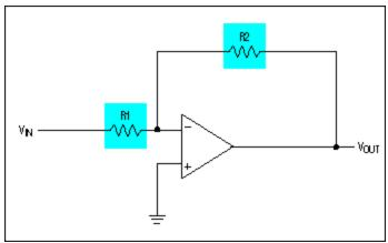
Figure 1. Fixed-gain inverting amplifier.
