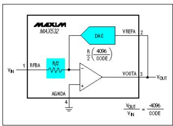
Figure 2. Programmable-gain amplifier.
