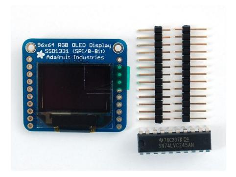
Since the OLED is 3.3V and also uses 3.3V logic, we need to use a logic shifter. We include a DIP logic shifter, the 74LVX245 with the OLED. If you're using a 3.3V logic
