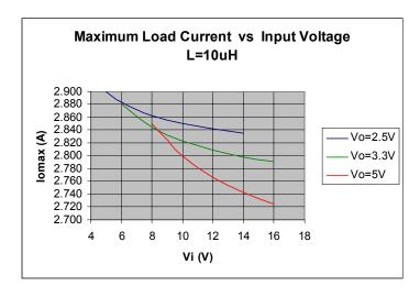
Figure 2. Theoretical maximum load current curves
