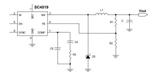
Figure 3. Compensation network provides 2 poles and 1 zero.
