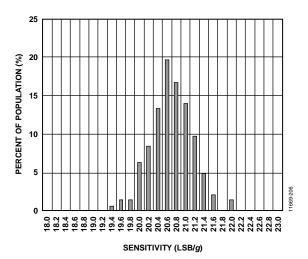
Figure 10. X-Axis Sensitivity at 25°C,  $V_S = 2.5 V$
