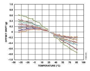
Figure 9. Z-Axis Offset Drift, 15 Parts Soldered to PCB,  $V_5 = 2.5 \text{ V}$
