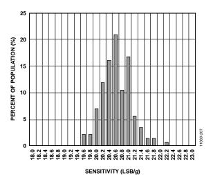
Figure 11. Y-Axis Sensitivity at 25°C,  $V_S = 2.5 V$
