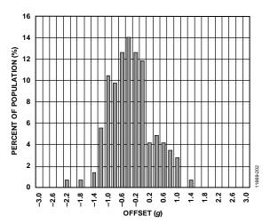
Figure 6. Z-Axis Zero g Offset at 25°C,  $V_5 = 2.5 \text{ V}$
