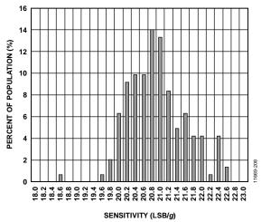
Figure 12. Z-Axis Sensitivity at 25°C,  $V_S = 2.5 \text{ V}$
