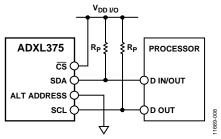
Figure 28. I<sup>2</sup>C Connection Diagram (Address 0x53)
