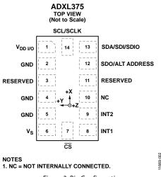
Figure 3. Pin Configuration
