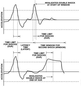
Figure 35. Shock Interrupt Function with Invalid Double Shocks
