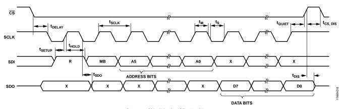
Figure 26. SPI 4-Wire Read Timing Diagram
