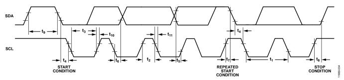
Figure 30. I<sup>2</sup>C Timing Diagram
