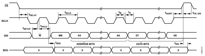
Figure 25. SPI 4-Wire Write Timing Diagram
