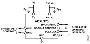
Figure 31. Application Diagram
