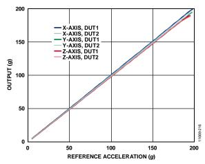
Figure 20. Output Linearity over the Dynamic Range
