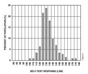
Figure 16. Z-Axis Self-Test Response at  $25^{\circ}$ C,  $V_{\text{S}} = 2.5 \text{ V}$
