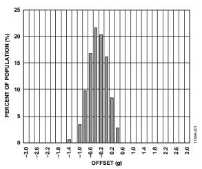
Figure 5. Y-Axis Zero g Offset at  $25^{\circ}$ C,  $V_{\text{S}} = 2.5 \text{ V}$
