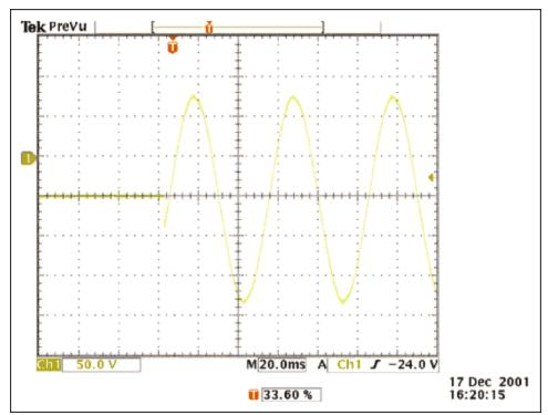
Figure 2. The ringer signal of a typical telephone exceeds 200V<sub>P-P</sub> (vertical scale is 50V/div).
