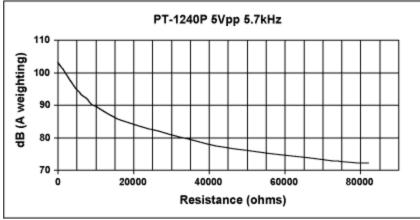
Figure 14. PT-1240P sound pressure vs. Rsource.
