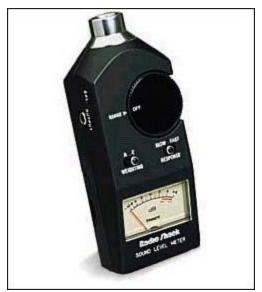
Figure 4. Radio Shack analog-display sound-level meter.
