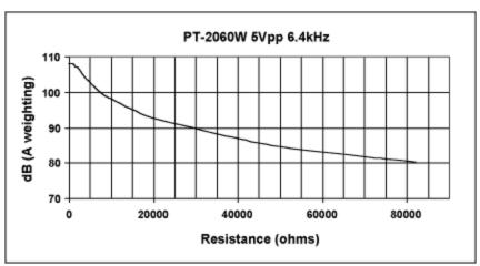
Figure 11. PT-2060W sound pressure vs. Rsource.
