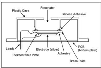
Figure 1. Cut-away view of audible PZT.
