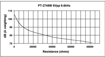
Figure 8. PT-2745W sound pressure vs. Rsource.
