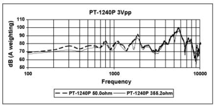
Figure 13. PT-1240P with 3V<sub>P-P</sub> excitation.
