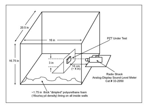
Figure 5. Sound pressure test setup.
