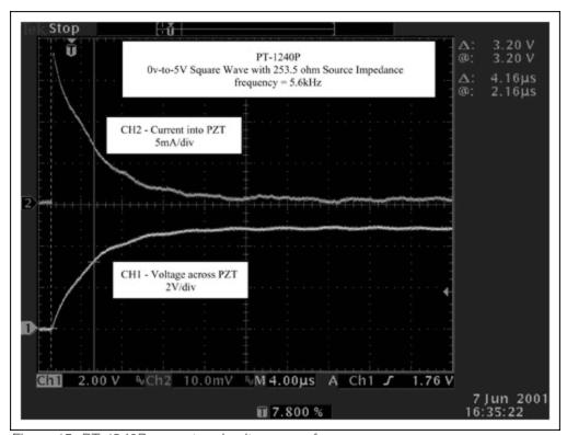
Figure 15. PT-1240P current and voltage waveform.
