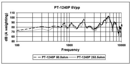
Figure 12. PT-1240P with 5V<sub>P-P</sub> excitation.
